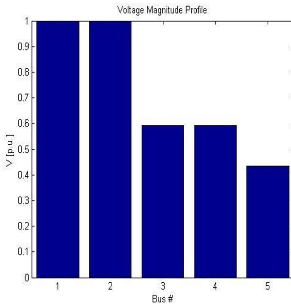
Fig-4: Voltage profile without DG connection
