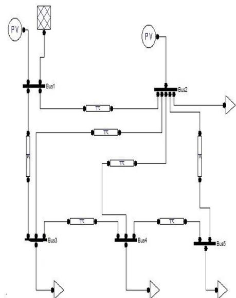
Fig-1: IEEE-5 bus network without DG connection
