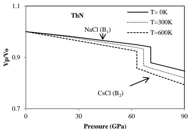
Figure 2. Variation of  $V_p/V_o$  with pressure
