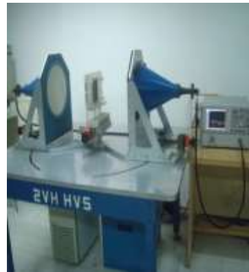
Figure 6.a. Experimental set up b. Schematic for free space measurement set up
