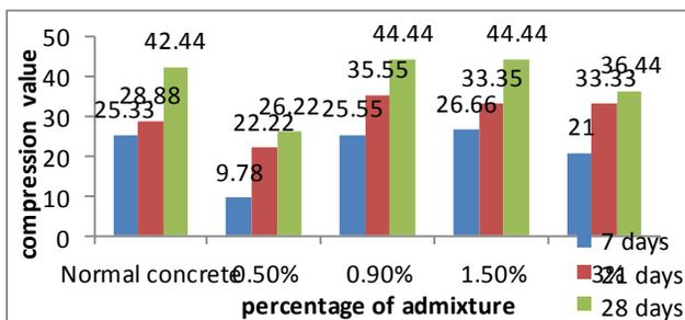
Figure 4 combined graph of compressive strength vs different percentage of admixture
