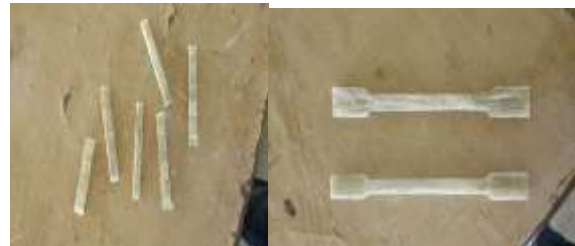
Fig. 2.4 Test specimens for izod and tensile test
